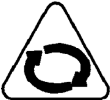
Hazard caused by continuous rotation
